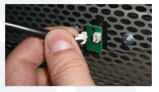
Carefully remove the cable attached to the led PCB assembly.
